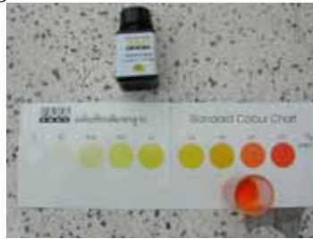
Figure 6: Use of chlorine test kit
